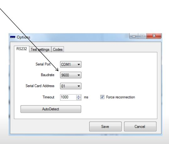
Serial Card Address: is the address of the device
