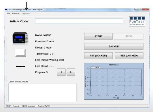
**Semaphore light**: GREEN if result is OK, YELLOW if the test is in progress, RED if the test is KO, WHITE if the result is ABORT of not determinated
