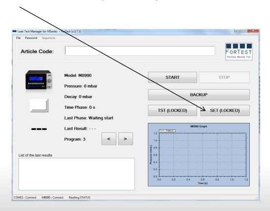
**GRAPH**: Graph the pressure and the decay during the test
