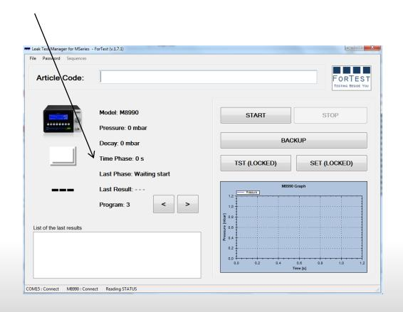
**Last phase**: is the last phase evaluated during the full cycle of test (for example : "Waiting start", "Filling", "Settling", "Test"
