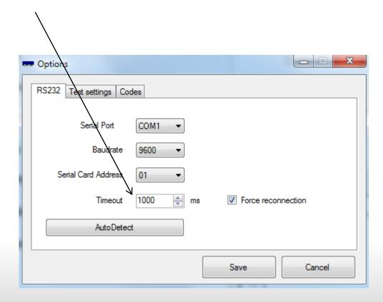
**Autodetect**: Perform a scan of the equipment on every serial port and if detected it automatically configure the connection with it
