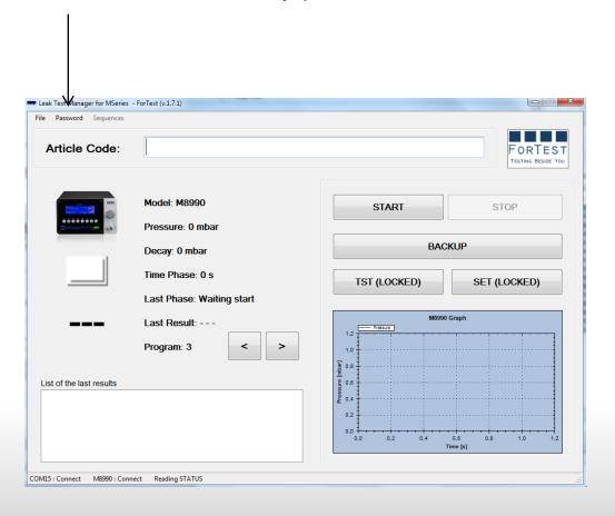
**Sequences**: create an association between an article code and the execution of automatic test of sequences. For example is it possible to read a barcode and automatically perform a test on the program 1, if result OK program 2, etc..
