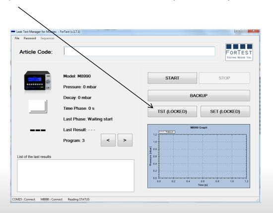
**SET**: Modify the setting parameters of the device If "LOCKED" it means that is password protected.
