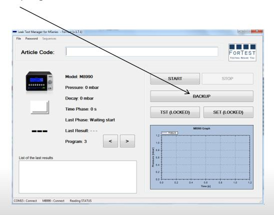
**TST**: Modify the testing parameters of a program (See "TST" for more informations) If "LOCKED" it means that is password protected.
