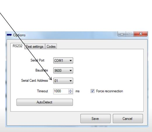
**Timeout**: If the software don't receive an RX answer in N-milliseconds it show a timeout error and the communication with the device is lost.
