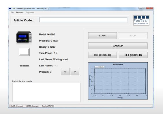
**Article code**: is the alphanumerical code that will be recorded into the test archive. It can be insert manually or via a barcode scanner (see options)
