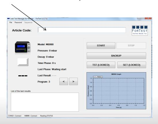
**Model**: is the model of the equipment connected.
