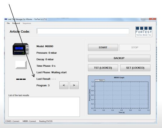
Program number: is the current program of test running on the device
